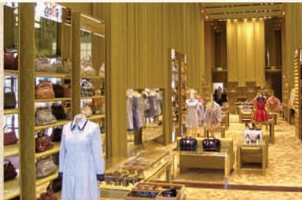
First Place -Keith Long-Quality Interiors, Corona, CA 60 yds of burlap backed acrylic-painted to look like metal, 700 yds of fabric on ceilings, soffits,walls, doors,panels,shelves and two 40 foot long molded fiberglass walls made to look like curtains- Prada's new flagship-Miu Miu on Rodeo Drive
